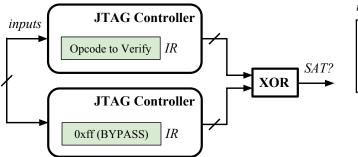
Fig. 3. Pairwise Opcode Comparison Equivalence Checking Formulation
