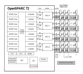
Fig. 6. OpenSPARC T2 SoC Architecture [25]
