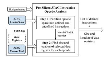
Fig. 2. Overview of Proposed JTAG Instruction Set Analysis Technique
