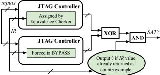
Fig. 4. Identifying Non-BYPASS Opcodes Using Counterexample Exclusion
